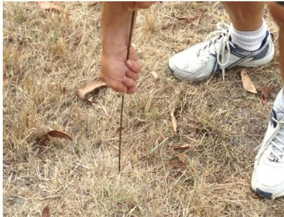
Home-made penetrometer for indicating soil compaction
