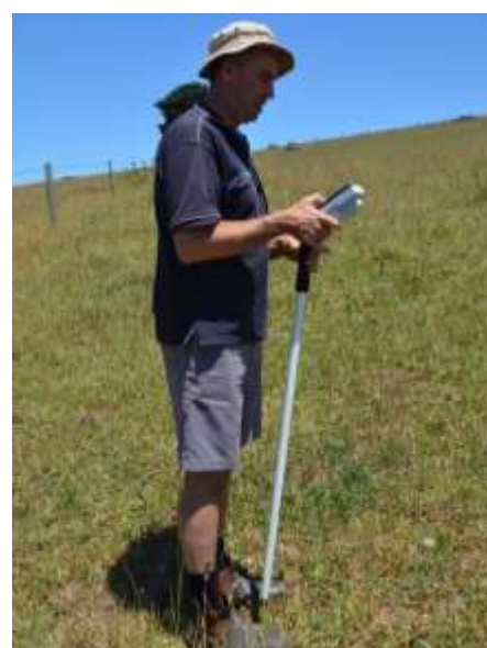
Figure 10: Measuring pasture growth with electronic pasture meter
